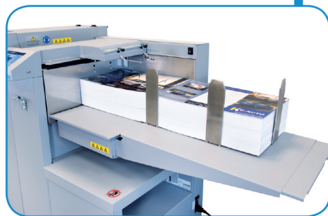
Extra long infeed table extends to hold media up to 51" in length
