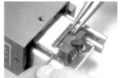
Installing the new springs
