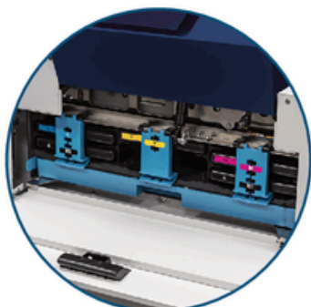
Clamshell Design Offers easy front access to ink tanks and the paper path
