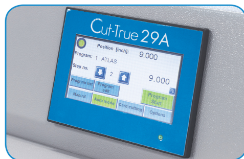
Full-color touchscreen control panel allows for programming up to 100 jobs
