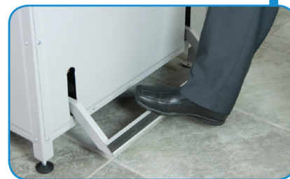
Foot pedal pre-clamp holds paper to check alignment prior to cutting
