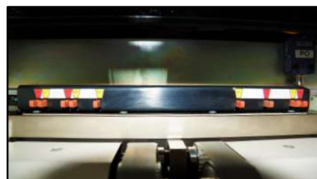
Wide range of quality punch dies with retractable pins
