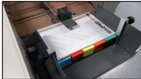
Adjustment of the feeder with magnetic and sliding stops
