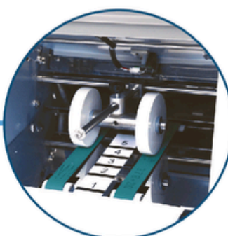
Output Conveyor & Stacker Wheels
