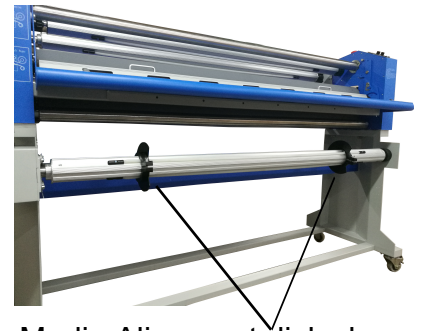
Media Alignment disks keep supply rolls from telescoping
