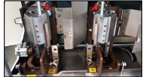
Quick and easy change of cutters with toggle clamping
