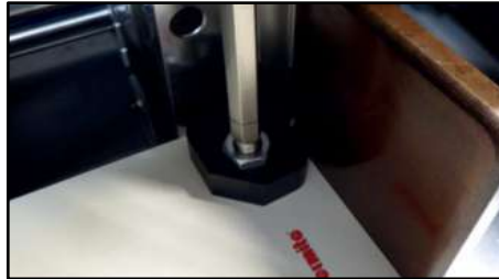
Document stack holding system for clean and precise cutting operations
