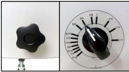
Locking/unlocking operation to a quick and simple adjustment according to the Wire-O® binding
