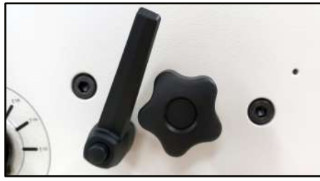
Many possible setups to adjust the parallelism of the press for a uniform closing of the Wire-O® binding
