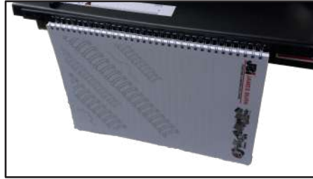
Hangers to facilitate the punching sheets insertion into the Wire-O® binding
