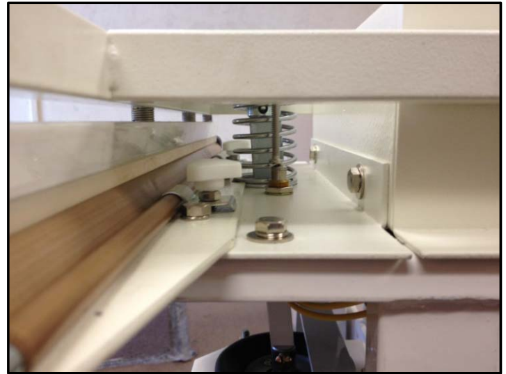
Figure 2. When jaw touches the base, the microswitch lever touches the actuator and there will be a “click” of the microswitch activation
