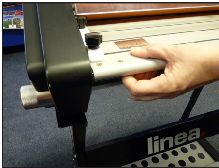
Remove the feed tray by retracting the bolt
