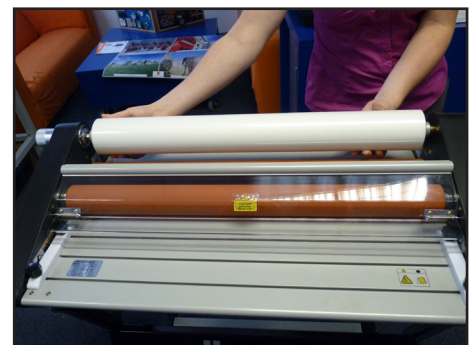
Refit the mandrel complete with the loaded film
