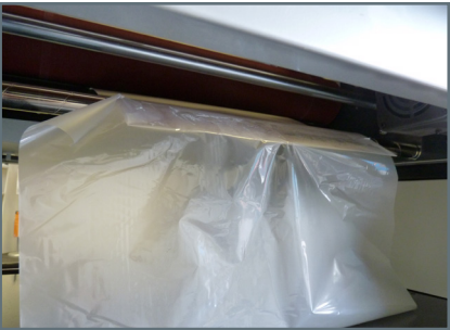
13. Tape bottom film to the feed card.
