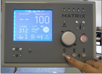
26. Push the forward button and select slow speed to load.
