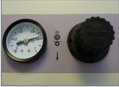
27. Adjust laminating roller pressure as required. Suggested pressure between 6-8 bar.
