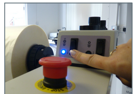
20. Press laminating roller switch. Roller will lower and light should illuminate.
